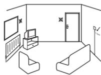
Care should be taken to mount the thermostat in a position which is not subject to direct sunlight or draughts. Preferably it should be mounted on an inside wall about 1.5m (5ft) above the floor in a position where it can respond to room temperature but away from the direct influence of radiators or other appliances giving off heat.
