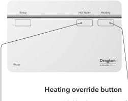
Pressing & holding the Heating button for >3s will turn on the heating for 2 hours. In this state the boiler will selfregulate its temperature. When the Heating override is active, the Heating LED will flash green. To turn off the override press the Heating button again. This will put the heating back under system control. Depending on the system settings the heating may stay on which will be indicated by a solid green LED.
