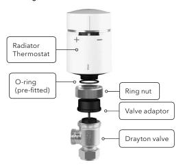
Place the small black plastic adapter serrated face down onto the valve. Position the metal ring nut over the black plastic adapter and screw it onto the valve. Now screw the Radiator Thermostat onto the black plastic adapter until tight. If the Radiator Thermostat is not facing the right direction, slacken the metal ring nut and rotate the Radiator Thermostat as required and re-tighten the metal ring nut.
