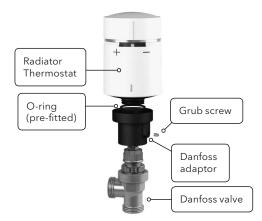
Slide the larger black plastic adapter small end first over the valve. Make sure that the hole containing the grub screw is facing away from you. This way, once its mounted, the markings of the Radiator Thermostat will be in the required position. Use an appropriate size Allen key to tighten the grub screw. Now screw the Radiator Thermostat onto the larger black plastic adapter until tight.
