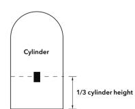
The plastic covered spring fixing cable should be cut to an un-stretched length of approximately 60-75mm (21/2"-3") less than the circumference of the cylinder and the hook and eyelet should be screwed into the ends. Stretch the cable round the cylinder, over the insulation, and position it in the groove across the front of the sensor housing, Engage the hook and
