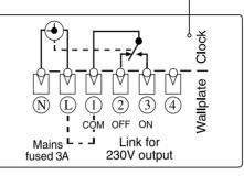
Connect the wiring as shown above
