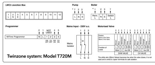
Make the wiring connections, as above, for the appropriate system. For surface wiring, snap out the cable entry strip on the bottom edge of the wall-plate. MiTime units are double-insulated and need no earth connection, but an earthing continuity (loop) terminal is provided for convenience.
