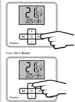
Press +/- to adjust +hr period between 0 and 3 hours Press (□) to confirm
