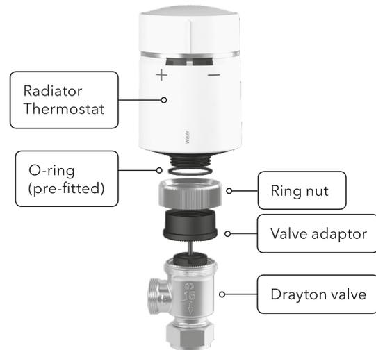
Place the small black plastic adaptor serrated face down onto the valve. Position the metal ring nut over the black plastic adaptor and screw it onto the valve. Now screw the Radiator Thermostat onto the black plastic adaptor until tight. If the Radiator Thermostat is not facing the right direction, slacken the metal ring nut and rotate the Radiator Thermostat as required and re-tighten the metal ring nut.
