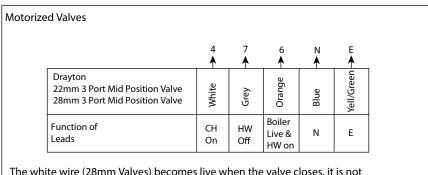
The white wire (28mm Valves) becomes live when the valve closes, it is not used and is wired to 'spare' terminals for sale isolation.
