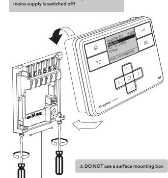
floor level, with reasonable lighting, good access, no condensation, no extremes of temperature and a supporting surface that fully covers the back of the unit. Position with 70mm clearance to the right, 25mm above and sufficient room to access the securing screws underneath. Fix, with terminals at the top, either direct to a flat wall using wall plugs and No. 6 x 1" (25mm) woodscrews, or on a flush mounting single conduit box type UA1 (BS4662) using M3.5 x 14 bolts.
