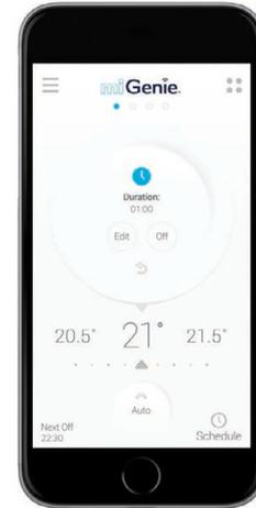
3. To adjust Boost temperature simply slide the set temperature left or right.
